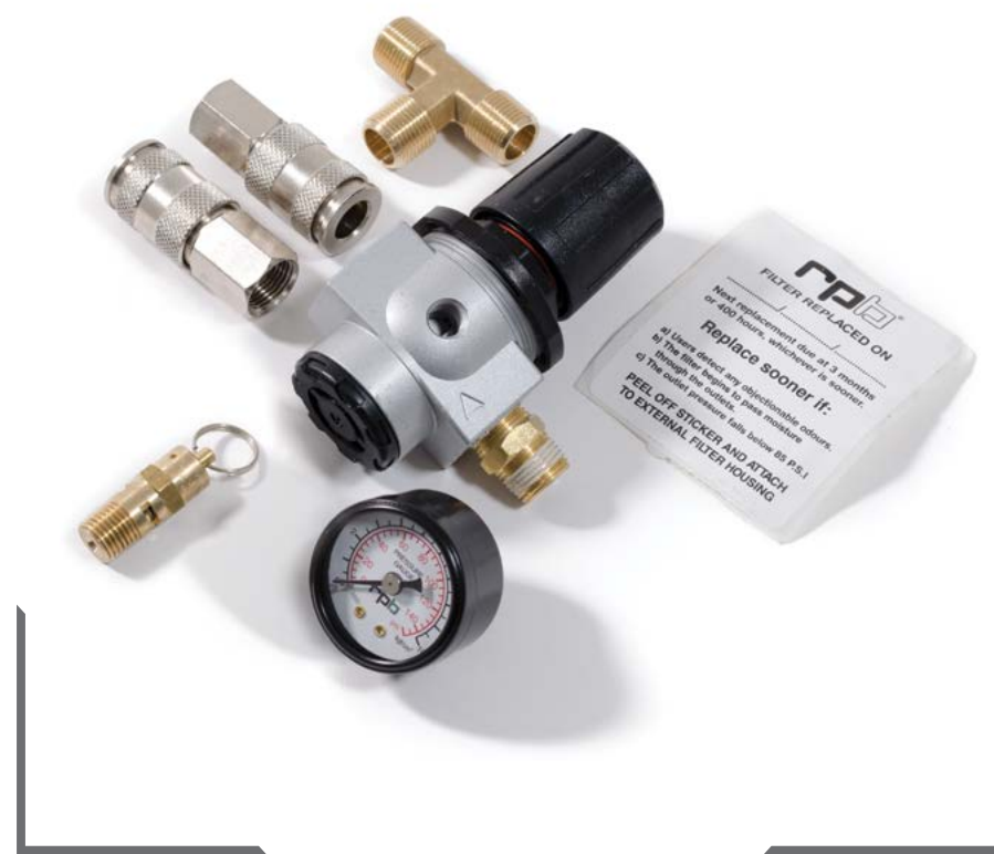
Parts Bag for Radex (04-900) (includes 2x 04-911 1/4" Coupler 3/8" FNPT, 04-912 3/8" Brass Tee, 04-914 Pressure Regulator, 04-915 Pressure Gauge, 04-916 Pressure Relief Valve, replacement date sticker) Part # 04-932
